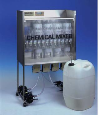
The mixing sequence is entirely conventional, taking water or processor overflow and adding chemical concentrates in turn. Each stage is checked, as if by a skilled technician and when correct, the mixer proceeds to the next step.
